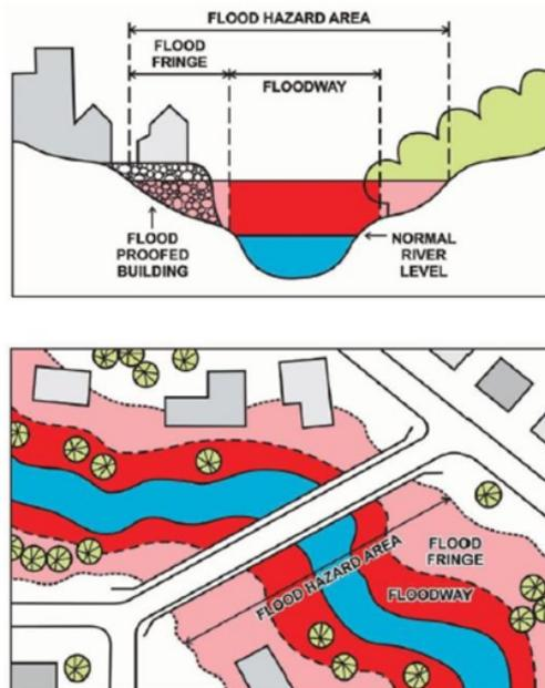
Illustration 2.5-4 - Flood hazard area, Floodway, and Flood Fringe
